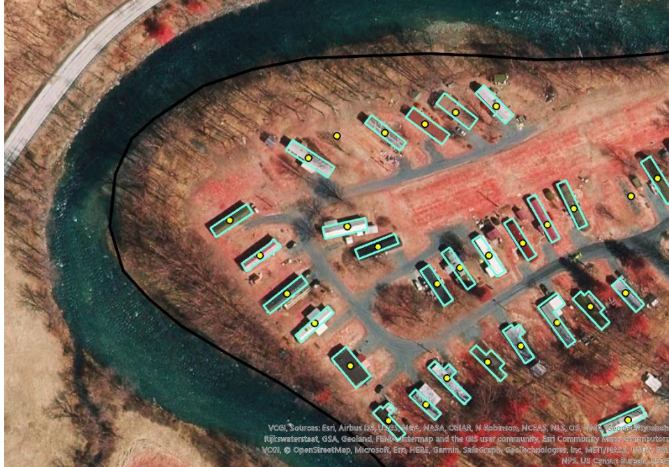
Figure 3. Buildings within MHC after correction of building footprints and updating. False color 2022 orthoimagery used as a reference layer is shown.
