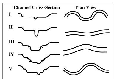
**Channel evolution process** showing channel down-cutting or incision in Stage II (cross-section), widening through Stages III and IV, and floodplain re-establishment in Stage V. Stages I and V represent equilibrium conditions. Plan view shows straightening and meander redevelopment that accompany cross-section changes. A flood-driven process taking place over decades.
