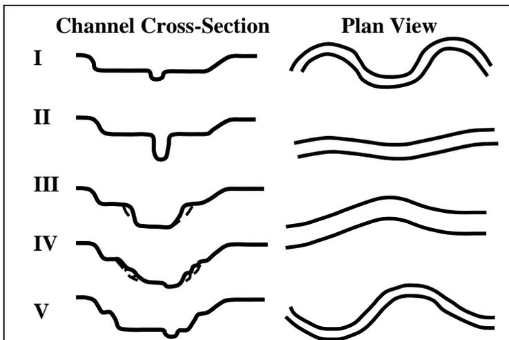
**Channel evolution process** showing channel down-cutting or incision in Stage II (cross-section), widening through Stages III and IV, and floodplain re-establishment in Stage V. Stages I and V represent equilibrium conditions. Plan view shows straightening and meander redevelopment that accompany cross-section changes. A flood-driven process taking place over decades.
